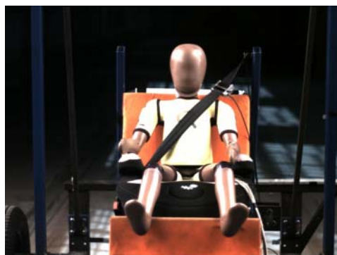
Typical shoulder belt routing before impact (belt is aligned with deflection sensor position)
