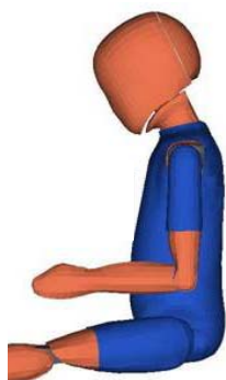
thorax shape from lateral view, slope of the thorax facilitates in addition to the shoulder design upwards movement of the shoulder belt
